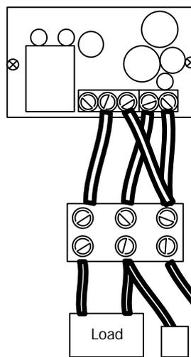
Attach the supplied 3-way connector block to the IntelliSwitch™ as shown.
